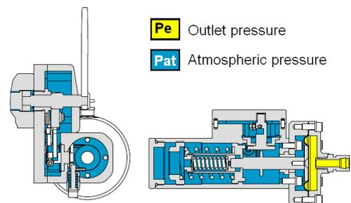
Figure 3 - SB 75 control device
