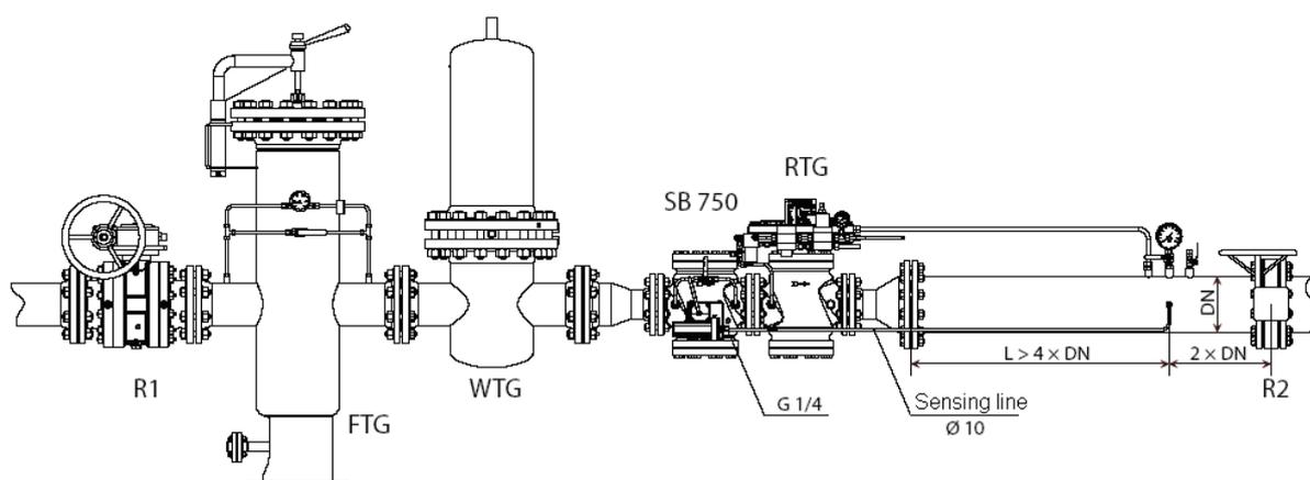
Figure 4 – Position recommended for installing
