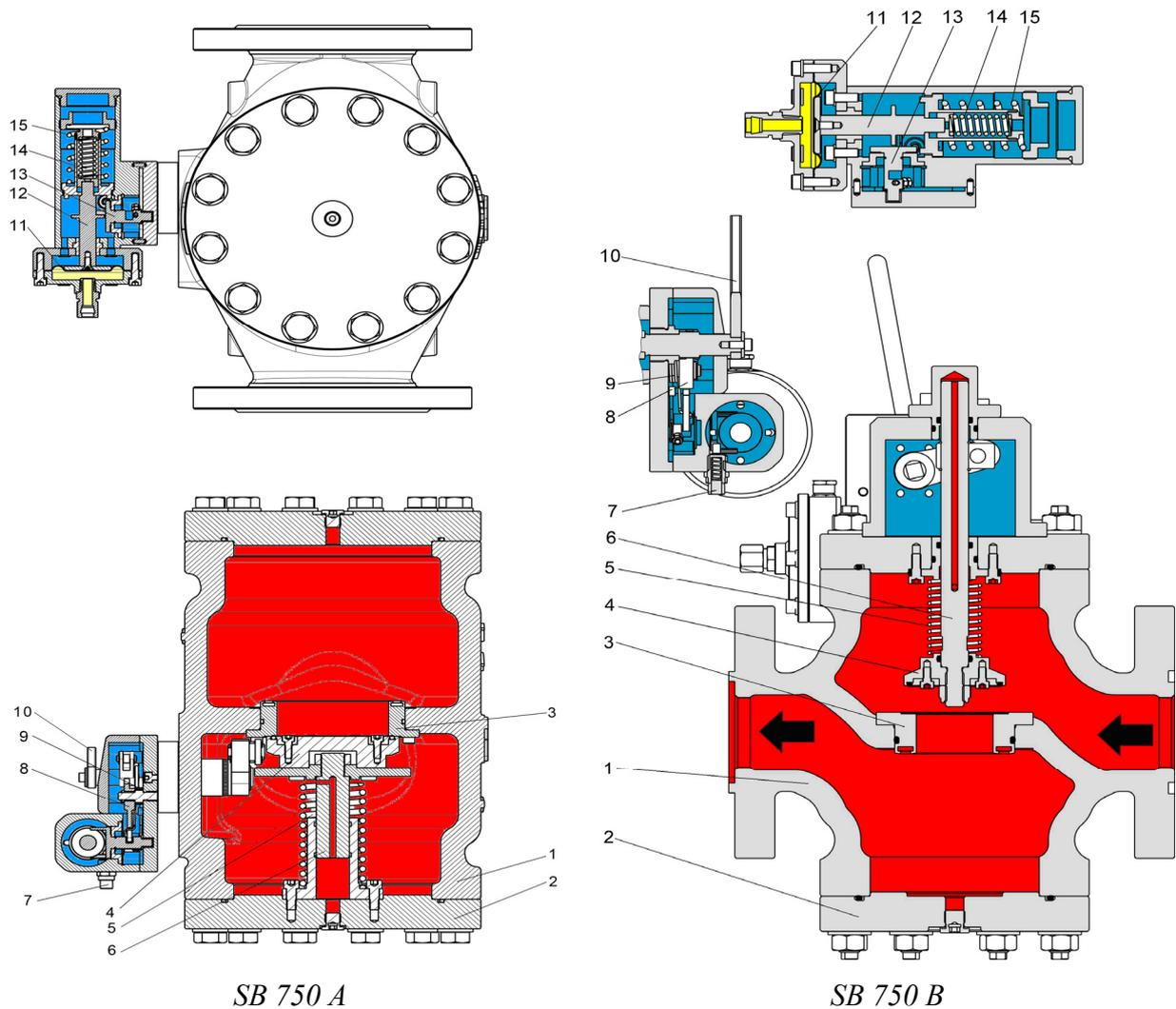
Figure 1 - SB 750 operating diagram
